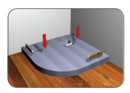
Place the Substrate Element into position and bed down onto the adhesive cement. Check that the Substrate Element is level in both directions using a suitable level.
