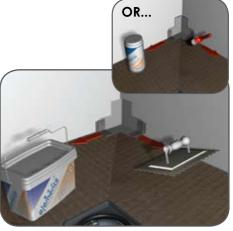
10. Place the Waterproofing Internal Corners into the internal corners of the shower area and push firmly into the tape sealer. Apply a further thin layer of tape sealer over the edges of the waterproofing internal corners.
