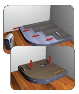
Spread board fixing adhesive across the surface of the Substrate Element. Lower the Shower Tray onto the Substrate Element and push firmly into position. Check with a level that the edges of the Shower Tray are level in both directions.
