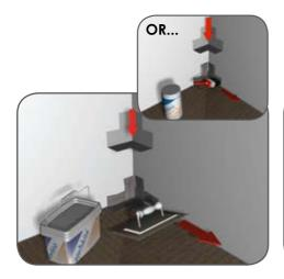
Note: Wear protective gloves, eye and breathing protection. Using the nonnotched end of the notched adhesive trowel, apply a thin layer of tape sealer to the internal corners of the shower area, slightly bigger than the pencil line marked in Step 8.
