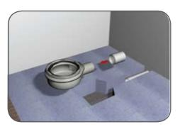
3. For water to drain away properly, the wastepipe must have a fall of at least 3cm per metre. The wastepipe must be properly supported to hold its own weight and that of the Shower Drain. Connect the Shower Drain to your wastepipe using a 2" solvent weld connector. Once the solvent weld has set, pour water down the drain to check that the waste is not blocked and that there are no leaks.
