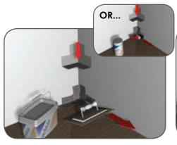
Note: Wear protective gloves, eye and breathing protection. Using the non-notched end of the notched adhesive trowel, apply a thin layer of tape sealer to the internal corners of the shower area, slightly bigger than the pencil line marked in Step 8
