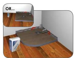
11. Where the shower area meets the wall apply a thin layer of tape sealer to the shower area and the adjoining wall approximately 60mm wide on both.
